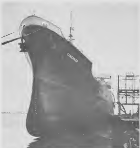
RIBING HIGH in the water with empty tanks, the Sangamon shoots off her bulbous-type bow which helps her attain a speed of 21 knots. This speed was well utilized when she was a U. S. Navy escort-type aircraft carrier during World War II.
